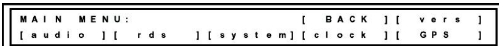
Main Menu (may only be accessed after entering a valid User Password or when no User Password has been set)
