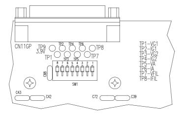
Because of the various tube type on which can be connected this card, can happen that the voltages measured, can be both positive and negative, but it's always necessary to have a positive voltage on the test point output. To obtain this, it is necessary to intervene moving some couple jumpers on the card on the ground of the negative value of the measure.
