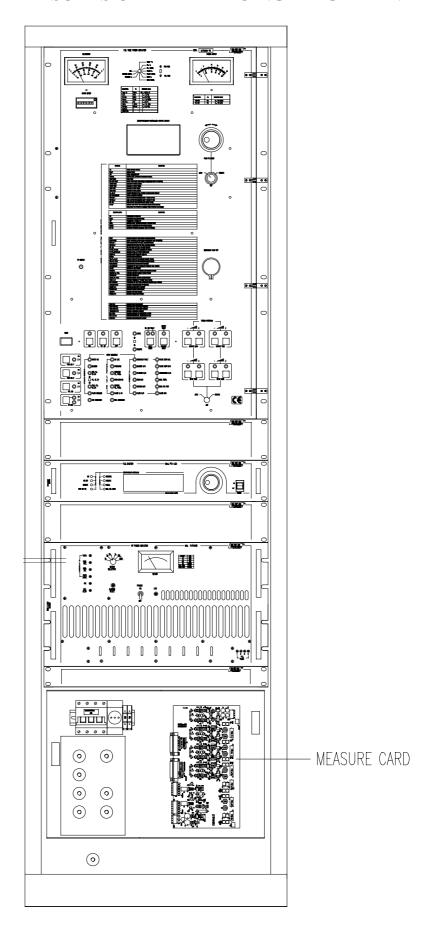
Before to proceed, check the test resistors values in according to the amplifier type that is used (in this case the type is VJ12000-TR that uses 3CX15000A7 tube, see as reference TABLE D and FIG. 39).
