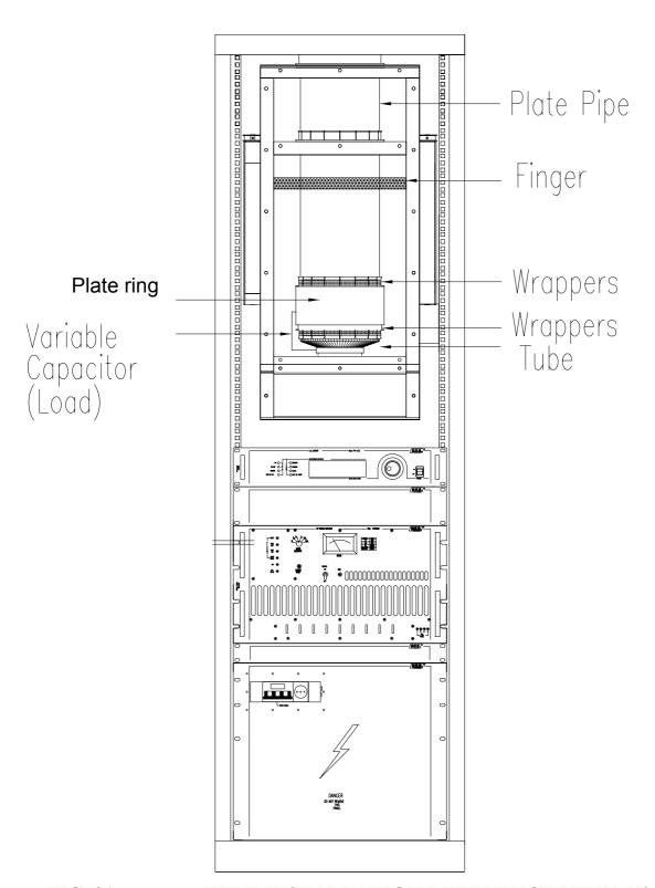
FIG. 21 TUBE INSTALLATION REFERENCE VIEW N°4
