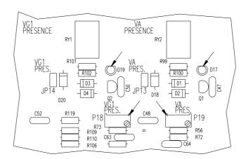
In case that on the equipment is installed a triode tube, the checking of the VG1 is excluded because this voltage is created automatically when the tube is in power and is created inserting the jumper JP14 to have a short circuit so that the starting sequence is ok, otherwise the equipment never go in high tension.
