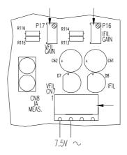
The filament current measure is obtained by a TA and then the voltage is included between 2.5Vac and 3.5Vac.
