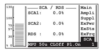
The PTX-LCDDSP has three subcarrier transmission inputs named SCA1, SCA2 and RDS. This menu shows the modulation level achieved by each input both in kHz and in percent. .
