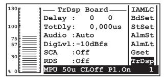
Delay Signal time delay setting, when used for isofrequency applications with poor step adjustment. The setting range for the first parameter is from 0 to 1900 steps of 5,25 μs each. The second parameter range is from 0 to 127 steps of 0,05 μs. The maximum time delay that can be set is 5.47 milliseconds. The actual time delay set is shown under item "Totdly"; it is expressed in microseconds up to a maximum value of 9981,35μs.
