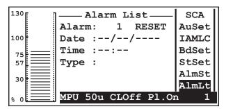
ALARMDisplay of stored alarm number. Select one of the six alarms as follows: select number and choose from the list of alarms 1 ... 6 using the encoder. Again using the encoder, move cursor to "RESET" and confirm reset operation to clear all stored events.
