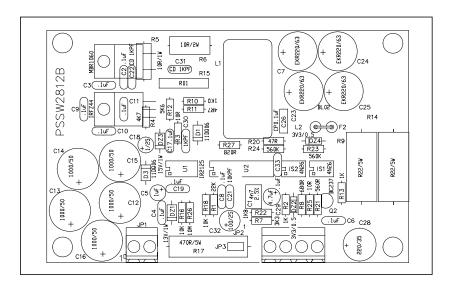
The second section consists in a card mounted on a heat sink located centrally in the machine. This card accommodates the power supply that feeds the different machine cards (audio, CPU...), a section that handles analogue inputs from the "Remote" connector and the automatic power level control system.
