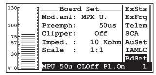
Mode Transmission mode selector: MONO, MPX\_U (unbalanced MPX BNC input), MBX\_B (balanced MPX XLR input), STEREO. The latter option is only enabled on the version with stereo coder.
