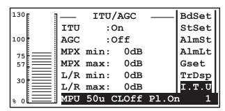
Enables automatic reduction of signal modulation energy according to standard I.T.U. 412. This feature is always given priority over the A.G.C. feature.
