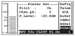
Pilot Add/remove pilot tone (convenient for some types of measurements). Chan.ph
