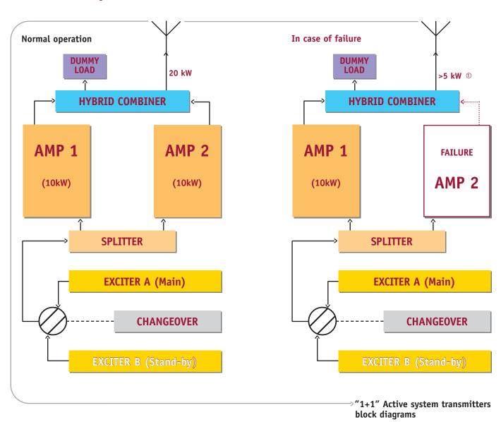
This system is composed of 2 combined amplifiers, A and B, connected to the antenna.
