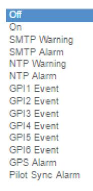
Pilot Sync Alarm: alarm starting when the frequency of the encoded RDS/RBDS signal is out of sync with an available external pilot(analogue MPX frequency / digital frequency by the SYNC/MPX inputs).
