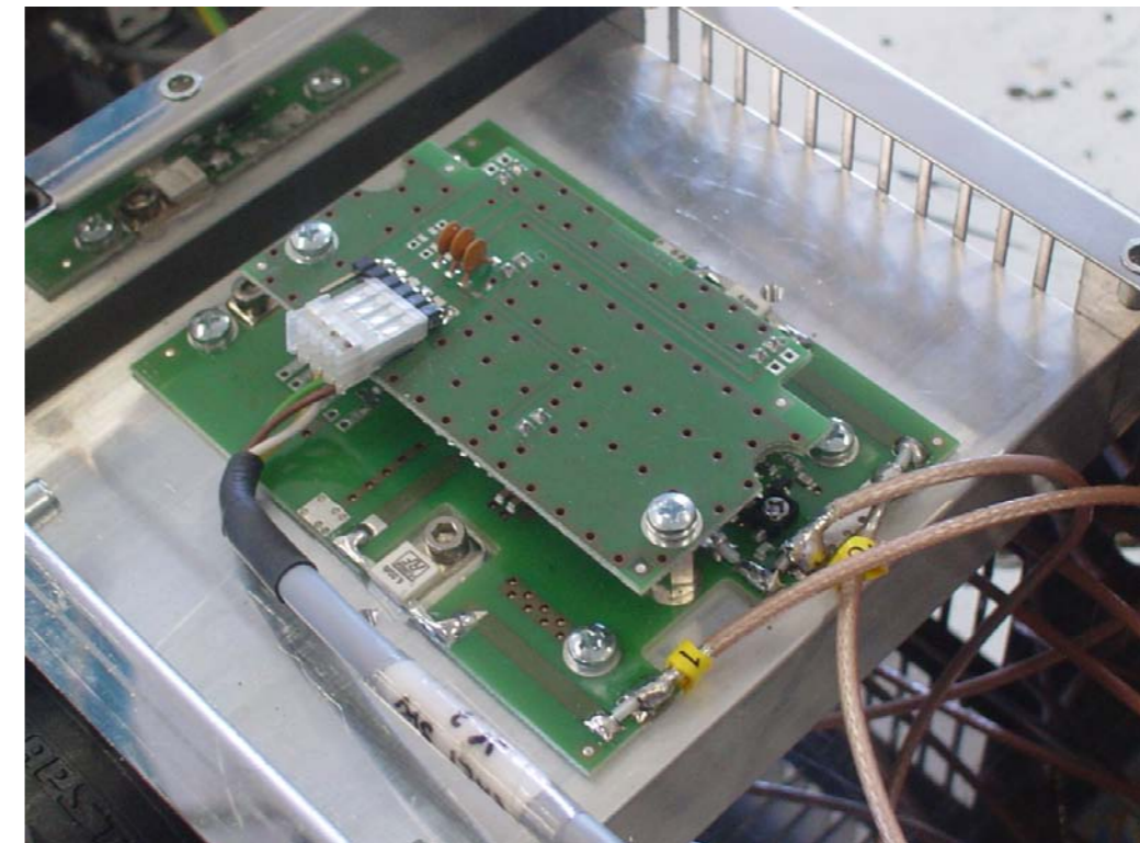
Exciter RF switch
