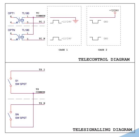
Schematic representation of TC/TS electromechanical interface operation
