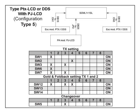
Figure 7.6: 1+1 GOLD system typical configuration for PTX LCD or DDS and PJ-LCD
