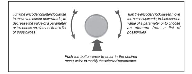
• **Rotation**: moves the cursor shows on the display; if you turn the encoder to the left (counter clockwise), the cursor moves downwards, if you turn it right the cursor moves upwards; it also permits to increase or diminish the parameters (turning the encoder left diminishes the parameter.
