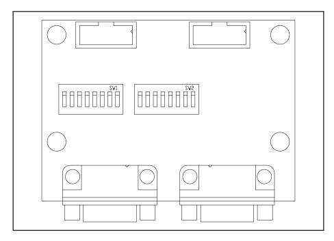
Figure 7.12: configurations of dip switch SW1 and SW2 for /V1 and /V4 versions
