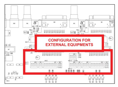
Figure 7.1: Dip-switch for external equipment configurations
